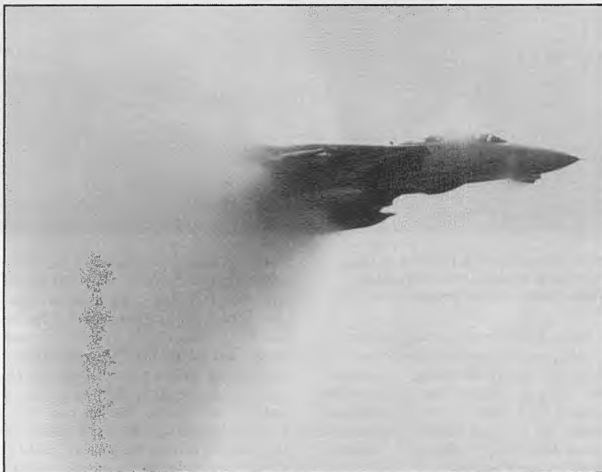
F-14 produces a vapor cone as it breaks the sound barrier. Photo: courtesy author
